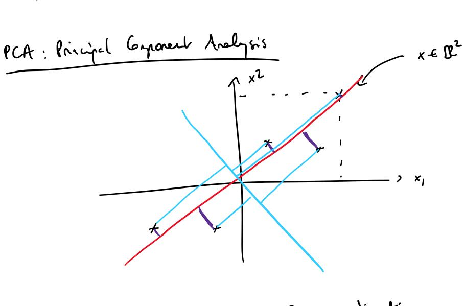
Reduce from 20 to 1D: Finds a direction (a vector we M2) onto which to project the data to projection error. So as to minimize the projection error. Reduce from ND to kD: Find a vectors  $u^{(i)}$ , ...,  $u^{(i)} \in \mathbb{R}^n$
